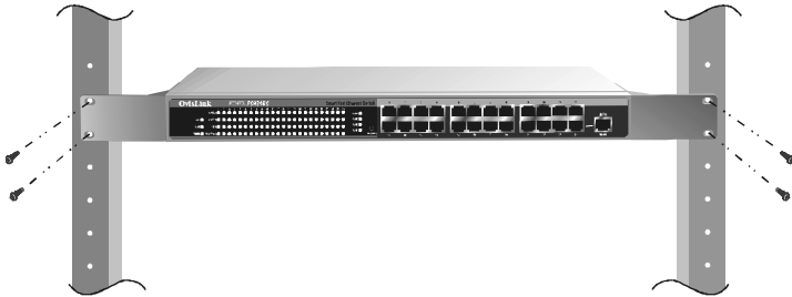
Fig. 3-3 Attaching the Switch to a standard-size rack
