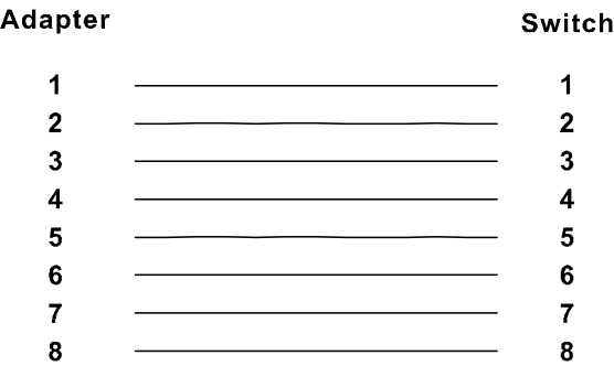
Fig 3-5 Pin assignments for straight-through cabling
